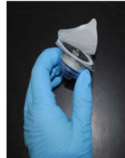
Grasp edges of filter cover, securing the filter between fingers, remove seal
