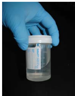
Cap sterile container, label, bag, and place in cooler on ice. Complete CoC and all field-related documentation
