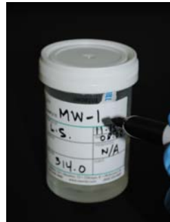
Cap sterile container, label, bag, and place in cooler on ice. Complete CoC and all field-related documentation
