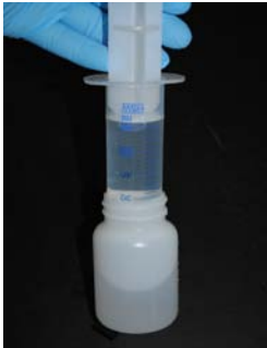
Completely fill syringe from non-sterile container
