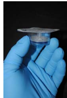
Grasp edges of filter cover, securing the filter between fingers, remove seal
