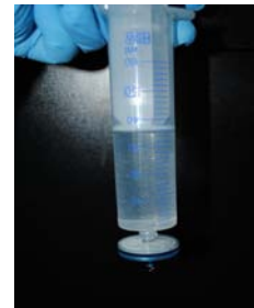
Turn syringe downwards, depress plunger gently, discarding the first 3-5mL
