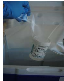
Cap sterile container, label, bag, and place in cooler on ice. Complete CoC and all field-related documentation
