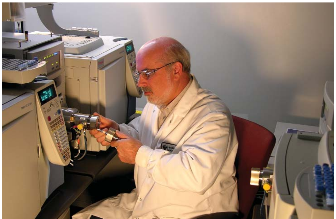
Principal chemist Nelson Risser changes ion volume to maintain optimal HRGC/HRMS instrument performance for PCB Congener testing.
