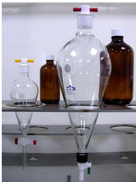
Reducing the volume used for organic extractions to 250 mL instead of the 1000 mL volume that was previously used softens the environmental impact of the method in several ways.
