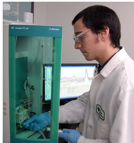
Clinton Wilson, instrumental water quality chemist, primes the ion chromatograph for low-level hexavalent chromium analysis.
