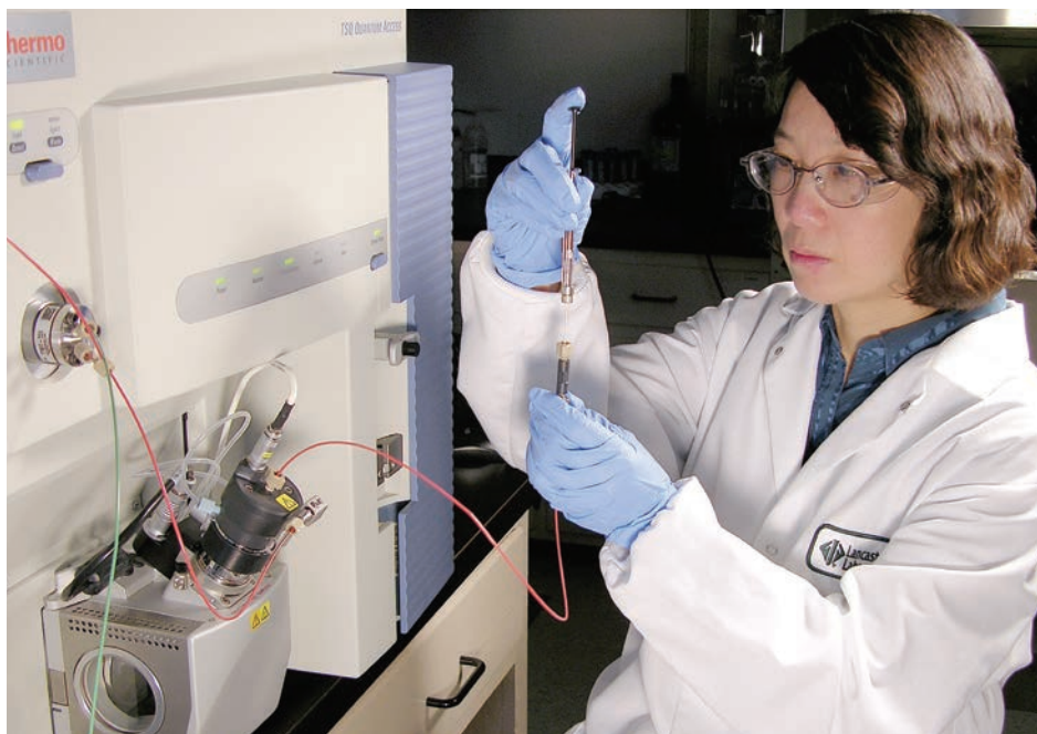
Analyst Meng Yu optimizes chromatography for a new client method using HPLC/MS/MS.
