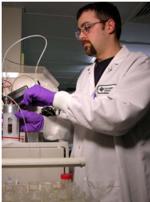
David Beck, chemist in the Metals Department, performs routine maintenance on the Agilent 7500ce. The instrument is equipped with an argon humidifier, which supplements the HMI and collision cell to allow for analysis of high matrix samples.
