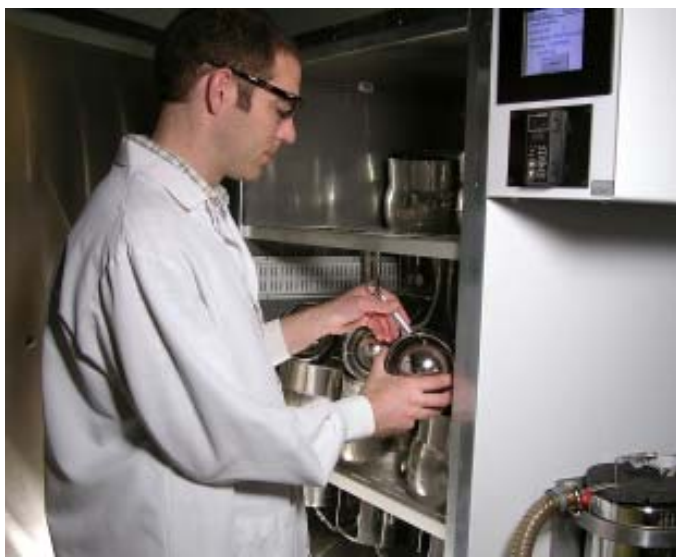
Jon Nardelli, senior chemist in the Volatiles in Air Department, utilizes the Summa canister system Lancaster Laboratories recently added, which decreases the time necessary to clean, certify and ship a Summa canister.
