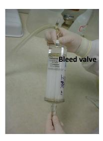
Adjust the flow rate to 2.0 L/min (0.5 G/min).
