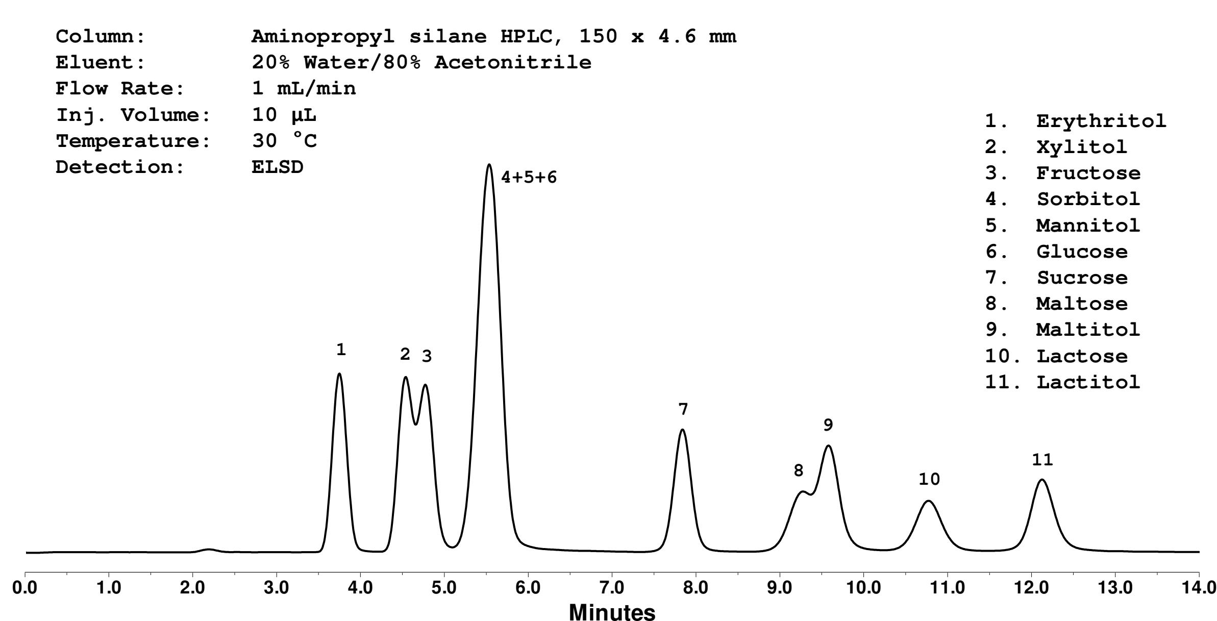
An efficient and reliable method has been developed to separate and analyze 5 sugars and 6 sugar alcohols within 20 minutes on a Waters Acuity UPLC (Ultra Performance Liquid Chromatography) system, using a Waters Acuity UPLC BEH Amide column.
