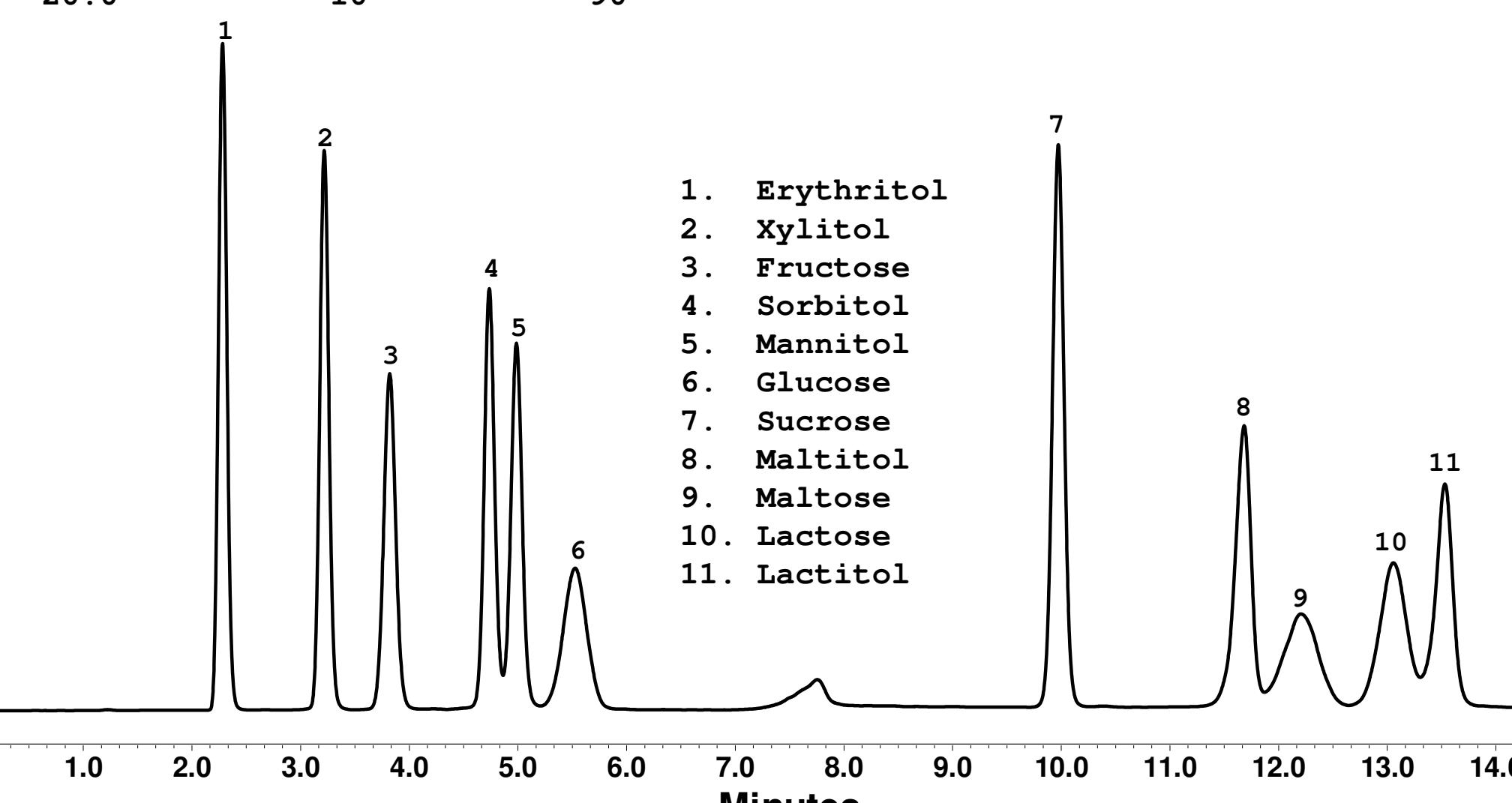
The elevated column temperatures and high pH values of the mobile phases (via addition of amine and ammonium hydroxide) help to suppress anomer formation from reducing sugars (glucose, maltose, and lactose), leading to relatively sharp peaks for those analytes.
